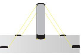
7B For substrates that prevent the use of pins/anchors, use dedicated weights or weight bags for lashing lines.
