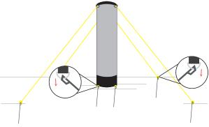
Fasten the pillar to the ground with straight pins. The lashing lines should be tensioned and stretched to their full length.
