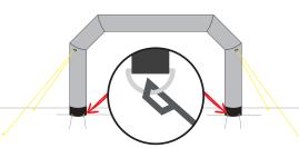
Put up and stabilize the gate using the lashing ropes. Fix the gate legs with pins to the ground.
