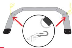
5 Pin the cables to the lashing eyes in the gate.
