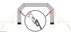
Fix the lines to the ground with pins. The lashing lines should be tensioned and stretched to their full length. For substrates that do not allow the use of pins/anchors, use dedicated weights for the lashing lines.
